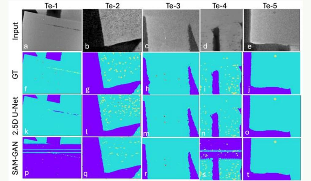
PEFT-SAM consistent across the different InD and OoD datasets. [Note: Even InD was real experiment, while training was on Synthetic data] Captures materials, pores, and inclusions for InD (Real) and weak OoD cases Struggles to recognize smoother material regions in strong OoD tasks.
