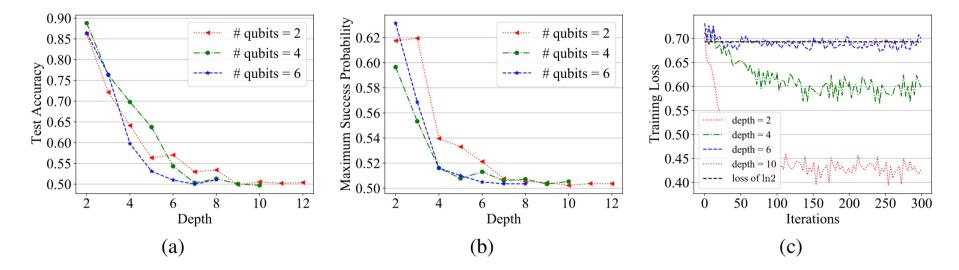
Figure 6: Numerical results for synthetic data sets under the encoding strategy in Fig. 4. In all qubit cases, (a) the test accuracy of QNN (or (b) the maximum success probability of POVM) will eventually decay to 50% or so with the depth growing; (c) In the 4 qubit case, for instance, the training losses of QNN do not decrease and stay at about  $\ln 2$  in the training process when the depth becomes large enough.
