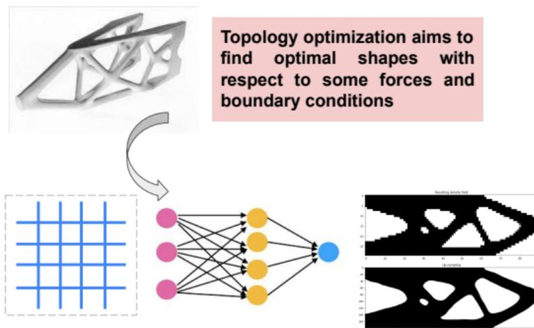
Topology optimization aims to find optimal shapes with respect to some forces and boundary conditions
